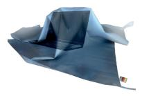
glass fiber fabric withstands temperatures of up to 1,000°C for short
